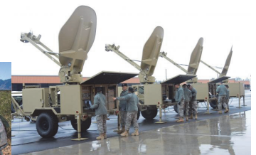
Satellite Transportable Terminals
